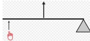
In a second class lever the input effort is located at one end of the bar and the fulcrum is located at the other end of the bar, opposite to the input, with the output load at a point between these two forces
