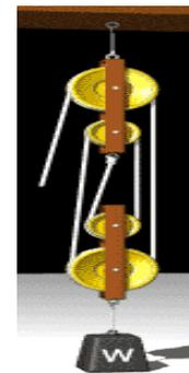
What is the **Mechanical Advantage** of this pulley system
